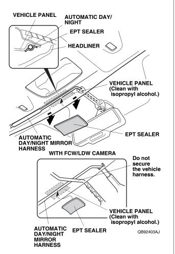
41. Secure the automatic day/night mirror harness to the vehicle panel with one EPT sealer as shown. Be careful not to crease the headliner.
