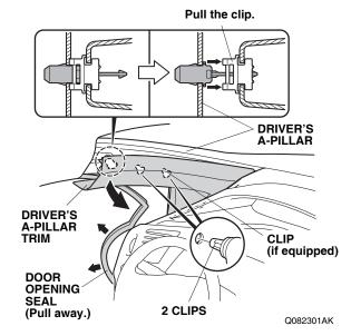
9. Pull out the driver's A-pillar trim to release the clips.
