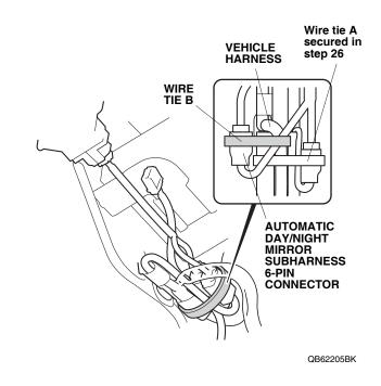
28. Using one wire tie B, secure the automatic day/night mirror harness 5-pin connector to the automatic day/ night mirror subharness as shown. Go to step 32.
