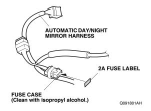
19. Attach the 2A fuse label to the fuse case on the automatic day/night mirror harness.
