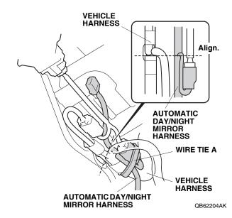
27. Using one wire tie B, secure the automatic day/night mirror subharness 6-pin connector to the vehicle harness as shown.
