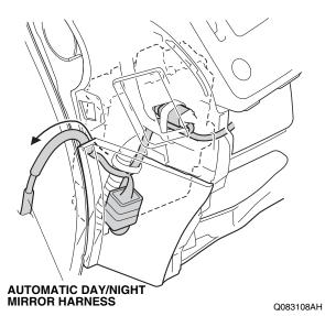
33. Insert the automatic day/night mirror harness between the dashboard and the driver's A-pillar.
