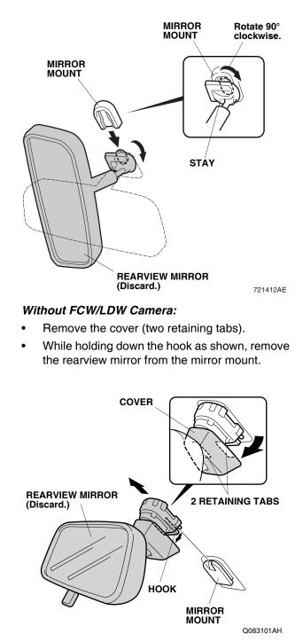
5. Wrap the end of a flat-tip screwdriver with tape. Locate the slot in the bracket cover, and insert a flattip screwdriver into the slot. Push the hook with the flat-tip screwdriver.
