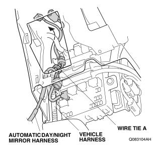
22. Using one wire tie A, secure the automatic day/night mirror harness to the vehicle harness.
