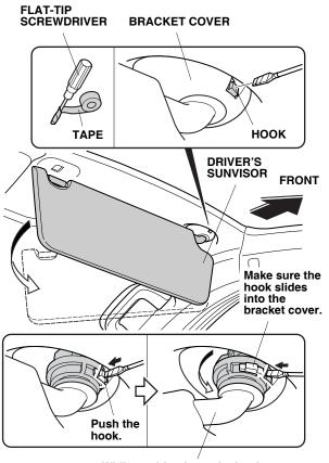
While pushing in on the hook, rotate the sunvisor backward <sub>Q090602BK</sub> about 45°.
