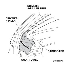
11. Remove the driver's A-pillar trim from the upper clip (unplug the vehicle connector, if equipped). Carefully remove the shop towel and any clips that fell from the driver's A-pillar trim.
