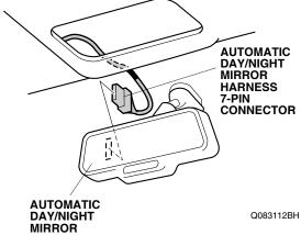
39. Align the green tape on the automatic day/night mirror harness with the headliner as shown. Route the automatic day/night mirror harness through the groove in the harness cover. Secure the harness cover to the automatic day/night mirror stay. Slide the harness cover inside the headliner.
