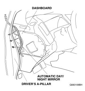
34. Align the green tape on the automatic day/night mirror harness with the vehicle clip, and secure the automatic day/night mirror harness to the vehicle harness with one wire tie A.
