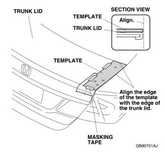
8. Using a felt-tip pen, mark the trunk lid through the two outboard in the template. Do not mark the inboard hole.
