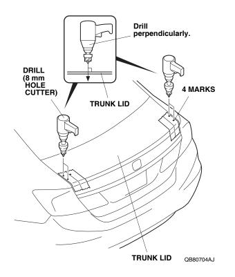
12. While wearing eye protection, drill a 10 mm hole at the remaining center-punched mark with a 10 mm hole cutter. Drill perpendicular to the trunk lid.
