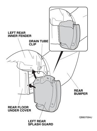
19. Secure the left rear splash guard with two 5 x 25 mm self-tapping screws and one 5 x 30 mm self-tapping screw in the order shown below.
