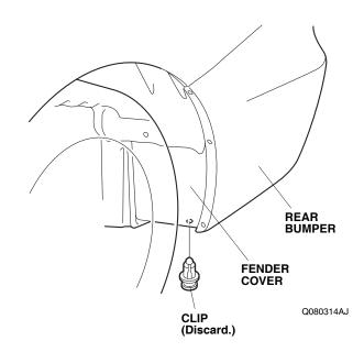
10. Pull the rear bumper away from the body, and release the seven retaining tabs.
