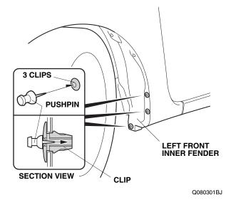
2. Using a pushpin, pierce the centers of the three clips shown on the left front inner fender.
