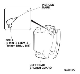
7. Remove any burrs from the edges of the hole with a file.
