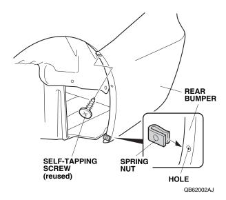
17. Install one spring nut over the hole in the rear bumper. Make sure to install the spring nut in the correct position and orientation.
