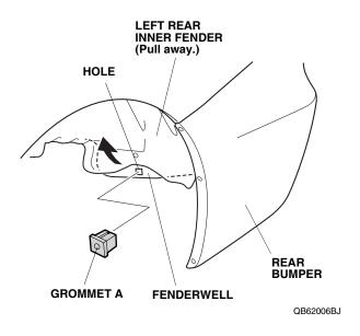
25. Pull the rear bumper away from the body, and release the seven retaining tabs.
