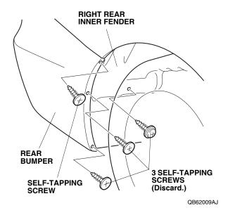
36. Working inside the fenderwell, use a small flat-tip screwdriver to release the tabs on the clip, then remove the clip with a trim tool. Remove the fender cover.
