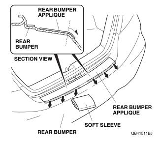
13. Using a shop towel, wipe away the excess 3M protective tape application solution. Allow the rear bumper applique to dry thoroughly.
