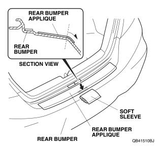
12. Use the soft sleeve to adhere the rear bumper applique to the lower section as shown.
