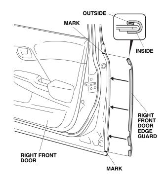
7. Starting at the character line, gently tap the right front door edge guard into position with a series of light taps using a rubber mallet, then work up and down. Make sure the position of the right front door edge guard is correct. Once in place, do not remove, reposition, or reinstall the right front door edge guard or it will not hold securely.
