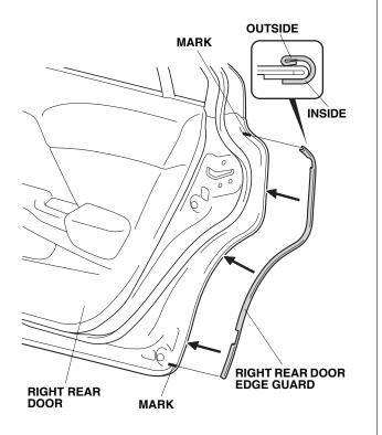
15. Starting at the character line, gently tap the right rear door edge guard into position with a series of light taps using a rubber mallet, then work up and down. Make sure the position of the right rear door edge guard is correct. Once in place, do not remove, reposition, or reinstall the right rear door edge guard or it will not hold securely.
