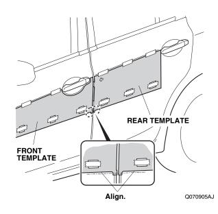
8. Using two alcohol wipes, clean the surface of both doors below the templates where the body side moldings will attach. Allow the alcohol to dry before installing the side moldings.
