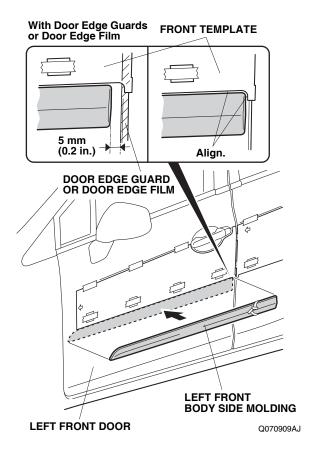
11. Press on the left front body side molding firmly with the palm of your hand while removing about 50 to 100 mm (2.0 to 3.9 in.) of the adhesive backing at a time.
