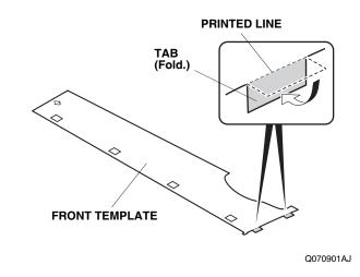
2. Align the two tabs on the front template against the rear edge of the left front door.
