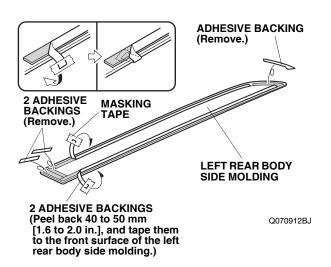
14. Align the edges of the left rear body side molding with the edges of the rear template, and attach the left rear body side molding to the left rear door.
