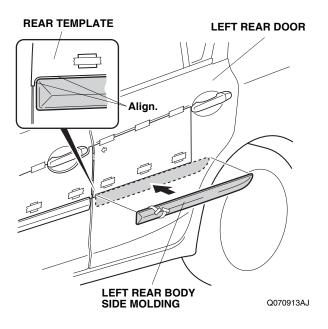
15. Press on the left rear body side molding firmly with the palm of your hand while removing about 50 to 100 mm (2.0 to 3.9 in.) of the adhesive backing at a time.
