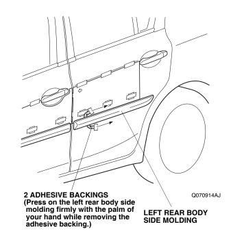
16. Using a rubber roller, apply firm pressure while rolling to set the adhesive. Apply firm pressure especially at the ends.
