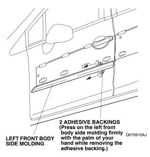
12. Using a rubber roller, apply firm pressure while rolling to set the adhesive. Apply firm pressure especially at the ends.
