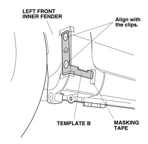
11. Using a felt-tip pen, mark the vehicle panel as shown.
