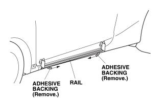
23. Carefully remove both templates A. Do not damage the templates. They are also used to install the right spoiler.
