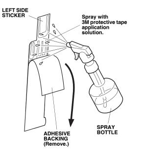
53. Spray the left side sticker with 3M protective tape application solution.
