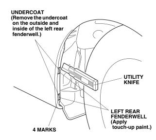
7. Apply touch-up paint to the area where the undercoat is removed, and allow it to dry thoroughly.
