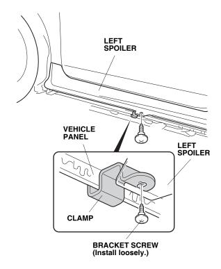
39. Assemble one screw and one washer-nut.
