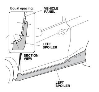
42. Remove the three adhesive backings in the order shown. Press the spoiler firmly against the vehicle panel with the palm of your hands to allow the adhesive to set.
