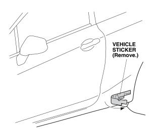
9. Using isopropyl alcohol on a shop towel, thoroughly clean the area where the left side under spoiler will attach.
