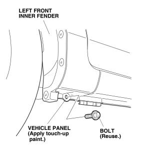
Apply touch-up paint to the area where the undercoat is removed. Allow it to dry thoroughly. 5. Using a felt-tip pen, mark the left rear fenderwell as shown.
