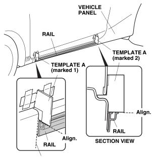
Align with the center of the template.
