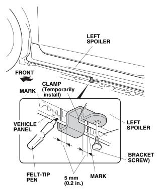
34. Using a felt-tip pen, mark the vehicle panel as shown.
