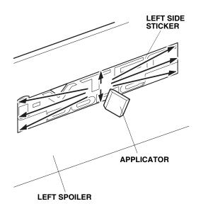
58. Use a shop towel to wipe the excess 3M protective tape application solution from the left side sticker. Allow the left side sticker to dry thoroughly.
