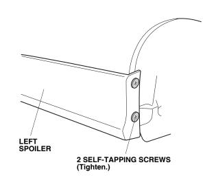
44. Tighten the bracket screw.
