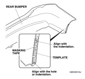
8. Using a pushpin, pierce the rear bumper at the hole in the template.
