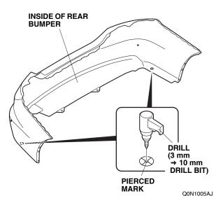
15. Using a file, remove any burrs from the holes.
