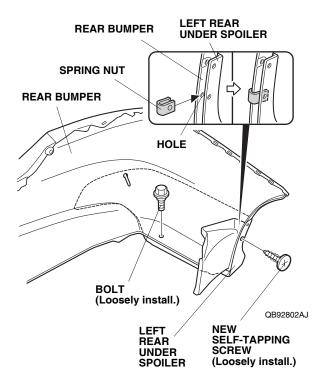
23. Loosely install a clip to the spoiler tab.
