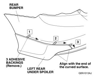
25. Remove three adhesive backings in the order shown. Press the left rear under spoiler firmly against the rear bumper with the palm of your hand for 30 seconds to adhere the left rear under spoiler.
