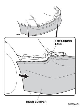
With the help of an assistant, remove the rear bumper (four retaining tabs). Place the rear bumper on a blanket to prevent damage.
