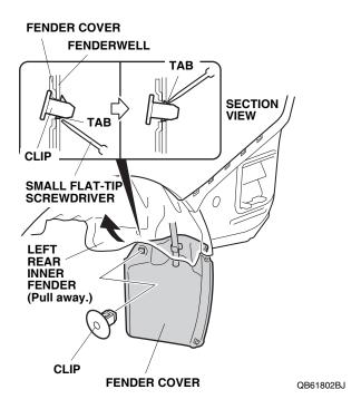
4. Remove the fender cover (one drain tube clip).
