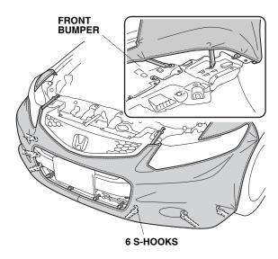
17. Route the elastic cord through eight loops on the bottom of the mask. Attach one S-hook to the bottom edge of the bumper on one side. Stretch out the cord after routing it through each loop, then attach the other S-hook to the bottom edge of the bumper on the other side.
