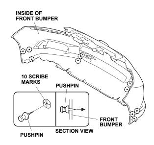
3. While wearing eye protection, drill the 10 pierced marks with a 3 mm drill bit, then enlarge the holes with a 10 mm drill bit.
