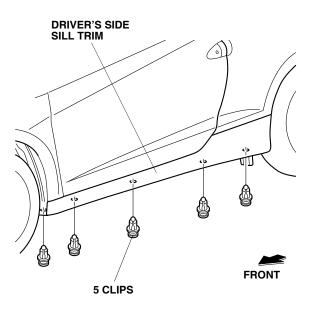
Remove the driver's side sill trim (nine clips). NOTE: Place the driver's side sill trim on a blanket after removal.
