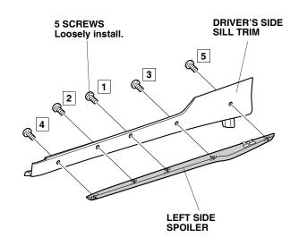
7. Using a utility knife, slit the adhesive backing on the left side spoiler at the location shown.
