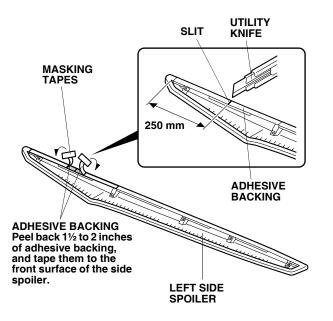
8. Peel back approximately 1½ to 2 inches of adhesive backing from each adhesive tape, and tape the ends to the front surface of the side spoiler.
