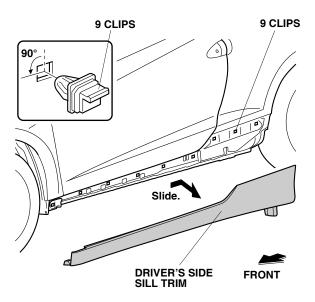
3. Remove the nine clips from the side sill trim by turning each clip 90° to remove.
