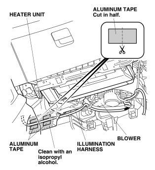
53. Using scissors, cut one aluminum tape in half. Secure the illumination harness to the back of the heater unit with two pieces of aluminum tape as shown.
