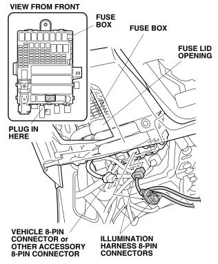
38. Plug the vehicle 8-pin connector into the illumination harness 8-pin connector. Go to step 41.
