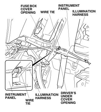
47. Route the illumination harness to the passenger's side of the vehicle as shown.
