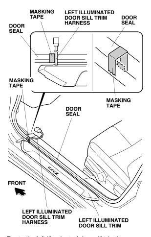
13. Route the left illuminated door sill trim harness over the door seal. Attach a piece of masking tape to the door seal to mark where the illuminated door sill trim harness crosses the door seal. 14. Pull up the door seal from the door sill trim at the masking tape.
