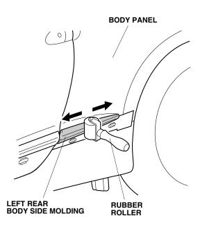
16. Turn the template over, and repeat steps 1 through 15 to install the body side moldings on the right side of the vehicle.
