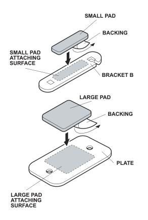
3. Using isopropyl alcohol on a shop towel, clean four plates where the large pads will attach. Remove the adhesive backings from the large pads and attach them to the plates.
