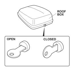
**Locking:** Press down on the lid. There should be an audible click. Be sure the lid is latched by attempting to lift the lid. Turn the key clockwise to lock the roof box. Make sure the strap ends don't dangle from the roof box.
