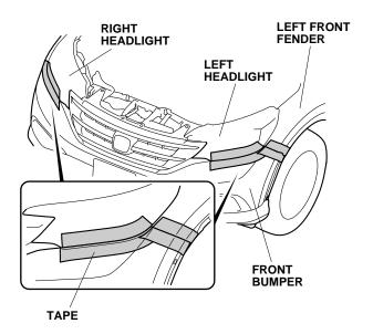
18. Apply masking tape to the front grille and front bumper.
