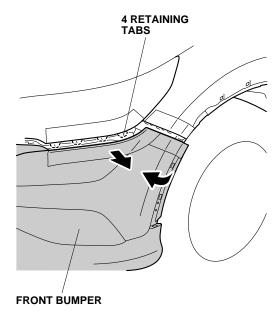
Apply masking tape to the front bumper.
