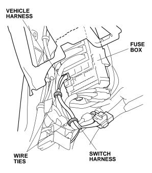
57. Unplug the vehicle connector from the light switch.
