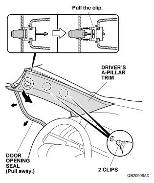
10. Pull out on the driver's A-pillar trim to release the clips.
