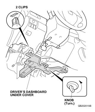
16. Remove the driver's dashboard lower cover (nine clips and unplug the vehicle connectors, if equipped).
