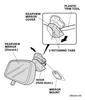
5. While holding down the hook, remove the rearview mirror from the mirror mount.
