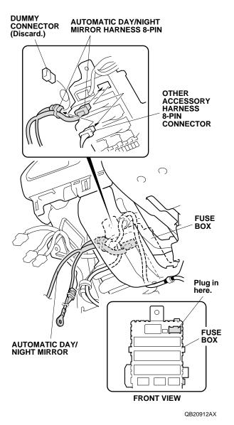
27. Route the automatic day/night mirror harness 7-pin connector out the square hole, and toward the outside of the vehicle as shown.
