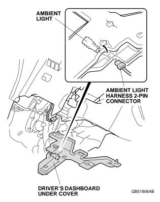
26. Plug the ambient light harness 2-pin connector into the ambient light, and reinstall the driver's dashboard under cover.
