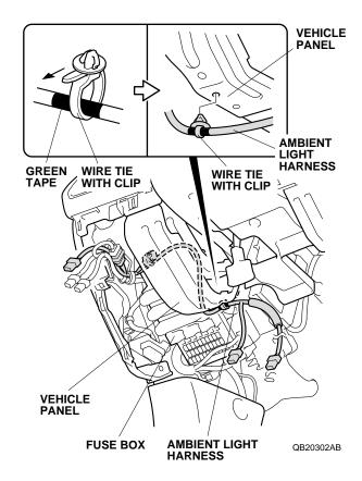
10. Using diagonal cutters, cut the clip portion off of one wire tie.
