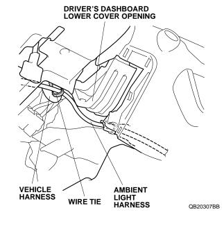
19. On the passenger's side of the vehicle, route and secure the ambient light harness to the vehicle harness with two wire ties.
