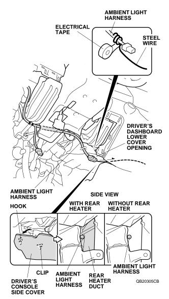
14. Attach a piece of steel wire to the ambient light harness with electrical tape. Route the ambient light harness through the center console from the driver's dashboard lower cover opening to the passenger's under cover opening. 15. Release the passenger's console side cover (two clips).
