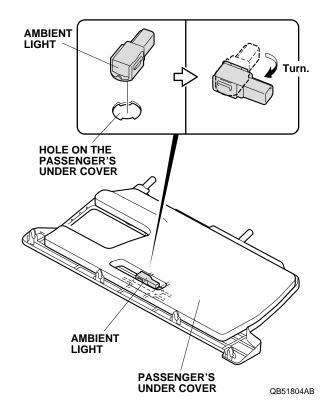
24. Plug the ambient light harness 2-pin connector into the ambient light, and reinstall the passenger's under cover.
