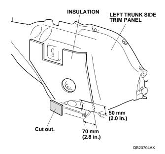
14. Attach the left template to the left trunk side trim panel with masking tape in the location shown.
