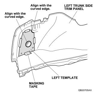
15. Using a felt-tip pen, mark the left trunk side trim panel through the hole in the left template. Remove the left template.
