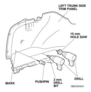
17. While wearing eye protection, drill the pierced mark in the left trunk side trim panel to 15 mm. First drill with a 3 mm drill bit, and finish with a 15 mm hole saw. Remove any burrs.
