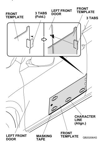
Insert the folded tabs of the front template into the opening between the front door and the B-pillar.
