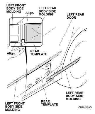
Make sure the edges of the left front body side molding and the left rear body side molding are aligned. 15. While applying light pressure against the left rear body side molding, carefully remove the taped adhesive backings. Remove about 50 to 100 mm (2.0 to 4.0 in.) at a time.
