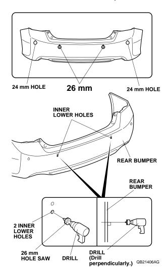
Using the sensor clips, install the two center sensors (Blue) into the 26 mm holes in the rear bumper. Note the direction and the pin location for each sensor.
