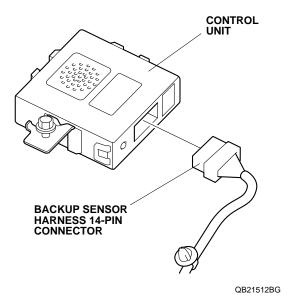
39. Secure the control unit to the vehicle panel with the flange bolt loosely installed in step 37 as shown.
