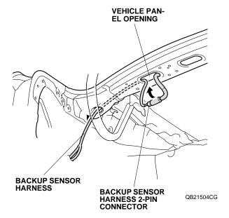
29. Secure the backup sensor harness to the vehicle harness with one wire tie.
