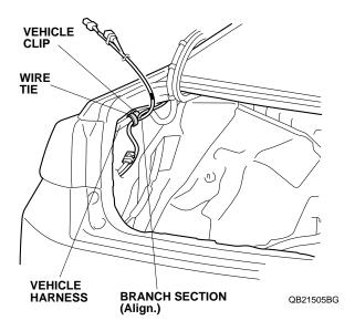
Align the green tape on the backup sensor harness with the vehicle clip, and secure the backup sensor harness to the vehicle harness with one wire tie as shown.
