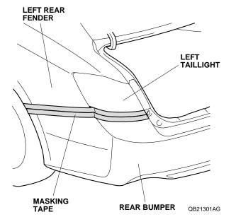
Remove the two bumper screws, four selftapping screws, and four clips.
