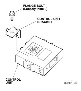
38. Plug the backup sensor harness 14-pin connector into the control unit.
