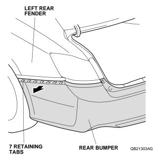
Release the three retaining tabs on each side of the bumper.
