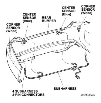
15. Secure the two subharness clips to the two center sensor clips as shown.
