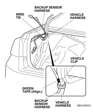
31. Secure the backup sensor harness to the vehicle harness with one wire tie.
