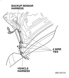
34. Unplug the vehicle 2-pin connector (Green) from the left taillight, and plug it to the backup sensor harness 2-pin connector.
