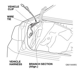
31. Align the green tape on the backup sensor harness with the vehicle clip, and secure the backup sensor harness to the vehicle harness with one wire tie as shown.
