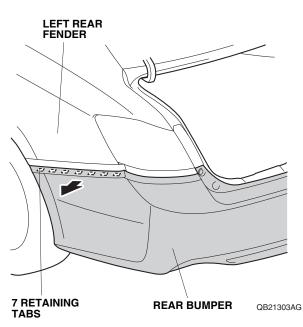
• Release the three retaining tabs on each side of the bumper.
