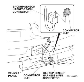
48. With the help of an assistant, bring the rear bumper next to the rear of the vehicle, plug the subharness 8-pin connector into the backup sensor harness 8-pin connector, and reinstall the rear bumper.
