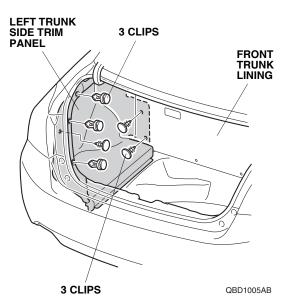
7. Pull away the weatherstrip, and remove the left trunk side trim panel. Remove the right trunk side trim panel the same way.
