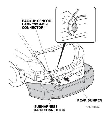
49. Check that all wire harnesses are routed properly and that all connectors are plugged in.
