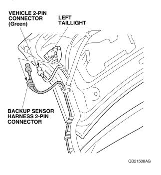
35. Plug the backup sensor harness 2-pin connector into the left taillight.
