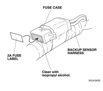
27. Route the backup sensor harness as shown, and plug the backup sensor harness 2-pin connector into the buzzer harness 2-pin connector.
