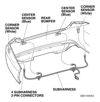
16. Secure the two subharness clips to the two center sensor clips as shown.
