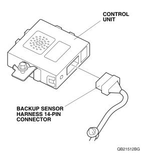
40. Secure the control unit to the vehicle panel with the flange bolt loosely installed in step 38 as shown.
