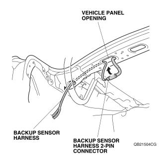
30. Secure the backup sensor harness to the vehicle harness with one wire tie.
