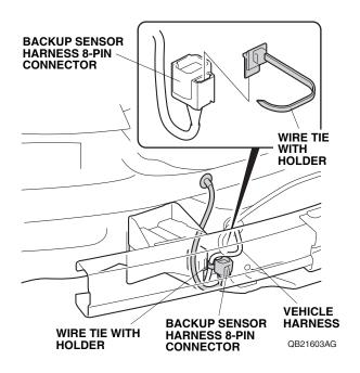
47. Install the connector clip to the backup sensor harness 8-pin connector, and secure it to the vehicle panel.
