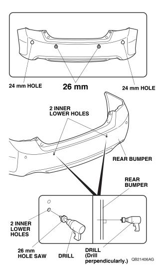
13. Using the sensor clips, install the two center sensors (Blue) into the 26 mm holes in the rear bumper. Note the direction and the pin location for each sensor.
