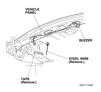
24. Using isopropyl alcohol on a shop towel, thoroughly clean the vehicle panel where the buzzer will attach.
