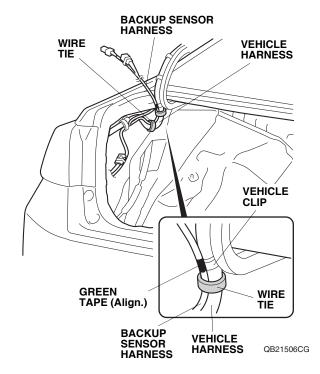
32. Secure the backup sensor harness to the vehicle harness with one wire tie.
