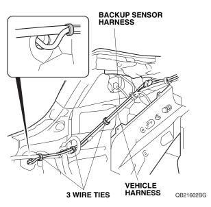
46. If equipped with vehicle harness, install the wire tie with holder to the backup sensor harness 8-pin connector, and secure it to the vehicle harness. Go to step 48.
