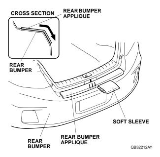
13. Repeat step 10 to smooth the left and right sides of the lower section on the rear bumper applique.
