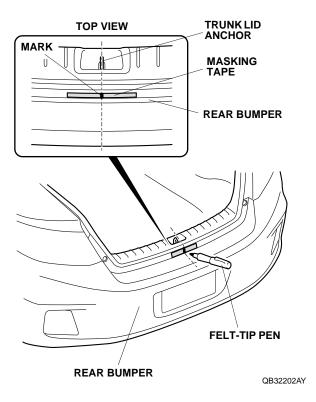
3. Align the rear bumper applique with the rear bumper and check the rear bumper applique position. Remove the rear bumper applique.
