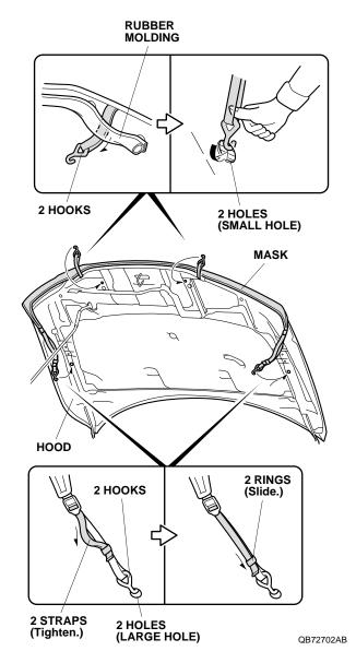
2. Route the two center hooks under the rubber molding, and attach them to each hole (small hole) on the hood.
