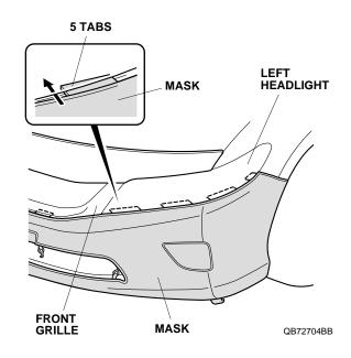
8. Pull the mask back toward the fenderwell, smooth out any wrinkles, and then snap the mask onto the snap-screw. Repeat on the right side.
