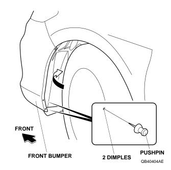
7. Thread a self-tapping screw into each pierced mark to make a hole in the front bumper. Remove the self-tapping screw.
