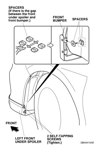
Turn the template over and repeat steps 2 through 17 to install the right front under spoiler on the right side of the vehicle.
