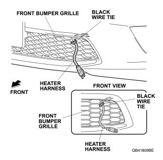
27. Install the protective cap to the front bumper grille and plug the heater harness connector into the protective cap.
