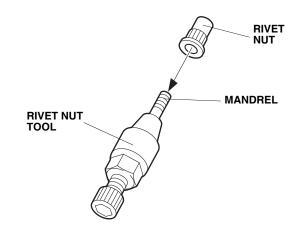
• Insert the rivet nut into the hole in the vehicle frame and install the hex wrench on the rivet nut tool.
