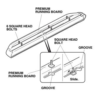
5. Position the premium running board onto the left brackets, align the square head bolts with the holes in the brackets and loosely install the six flange nuts. Do not tighten the flange nuts at this time.
