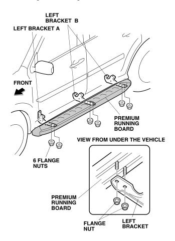
Center the premium running board on the left side of the vehicle, and tighten the six flange nuts loosely installed in step 5. Torque the flange nuts to 27 N·m (19 lbf·ft).
