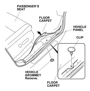
28. Remove the vehicle grommet from the floor.
