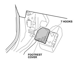
6. Remove the footrest (two flange nuts).
