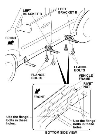
12. Position the left running board on the left bracket A and the two left brackets B. Install the left running board with six flange nuts. Do not tighten the flange nuts yet.
