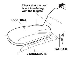
Open the roof box. Slide the plate forward or backward until the holes in the plate are over the front roof rack crossbar. The plate is located near the front of the roof box.
