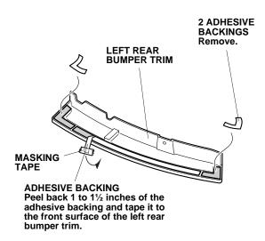
20. Align the edge of the left rear bumper trim with the curved edge of the rear bumper as shown. Attach the left rear bumper trim to the rear bumper.
