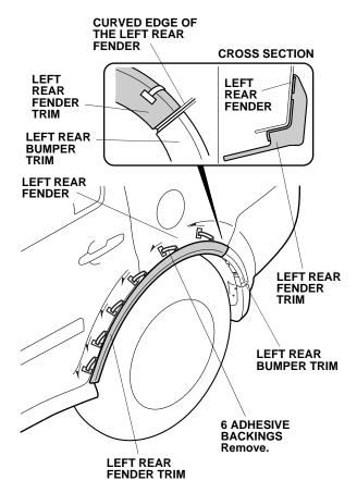
25. While applying light pressure against the left rear fender trim, carefully remove the taped adhesive backings.
