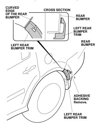
21. While applying light pressure against the left rear bumper trim, carefully remove the taped adhesive backing.
