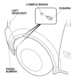
2. Slide the two spring nuts over the two small holes made in the front bumper.
