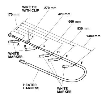
8. Using a white marker, mark the heater harness at each measurement shown.
