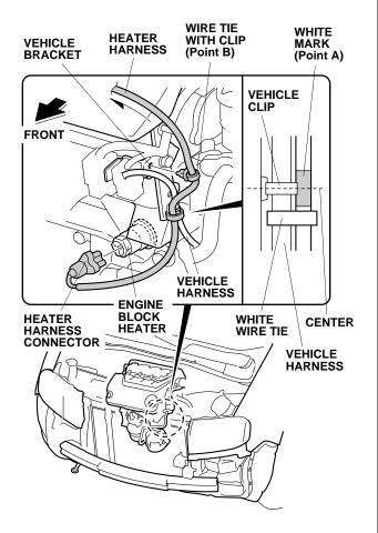
Route the heater harness up, and secure it to the vehicle harness with one white wire tie (Point A).
