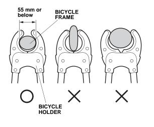
10. Position the bicycle on the channel. Lift the arm up, and clamp the holder around the bicycle's frame by pushing down the slider.
