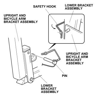
4. Slide the lower bracket assembly into the trailer hitch receiver until the hole in the bracket lines up with the receiver hole. Install the 12 x 40 mm bolt with a lock washer and a 12 mm washer through the receiver hole. Tighten the bolt securely.
