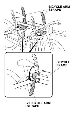
4. Install the two anti-sway straps and tighten each anti-sway strap securely around the bicycle frame.
