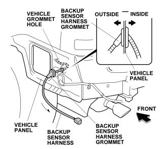
41. Slide the connector clip onto the backup sensor harness 6-pin connector, then install the connector clip into the vehicle panel hole.
