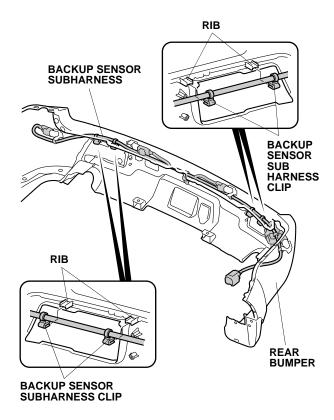
61. Secure the clip on the backup sensor subharness to the hole on the rear bumper as shown.
