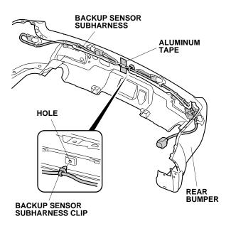
62. Using isopropyl alcohol on a shop towel, clean the rear bumper where the aluminum tape will attach. Secure the backup sensor subharness to the rear bumper with one aluminum tape.
