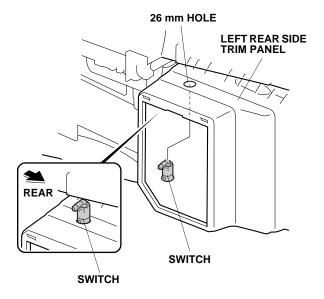
48. Using isopropyl alcohol on a shop towel, clean the switch bracket where the cushion tape will attach. Attach the remaining piece of cushion tape (from step 27) to the switch bracket as shown.
