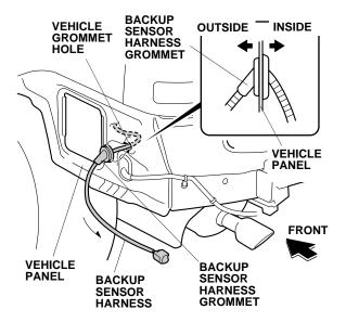
44. Slide the connector clip onto the backup sensor harness 6-pin connector, then install the connector clip into the vehicle panel hole.
