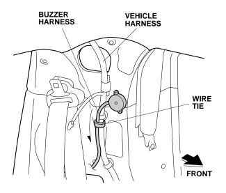
28. Continue routing the buzzer harness down along the vehicle harness, and secure it to the vehicle harness with three wire ties.
