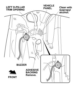
Route the buzzer harness along the vehicle harness, and secure it to the vehicle harness with one wire tie.
