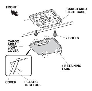
5. Remove the two bolts from the cargo area light case.
