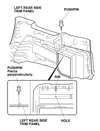
49. While wearing eye protection, drill a 3 mm hole at the pierced mark. Enlarge the 3 mm hole to 26 mm using a 26 mm hole saw. NOTE: Make sure to drill perpendicularly to the left rear side trim panel.
