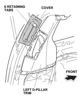
16. Using a rubber mallet wrapped with a shop towel, gently tap the left D-pillar trim at the area shown to release the clip.
