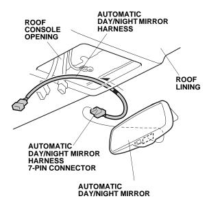
10. Align the green-tape on the automatic day/night mirror harness with the edge of the roof lining.
