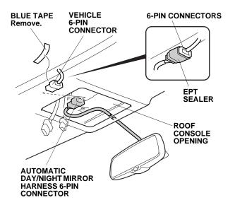
12. Wrap an EPT sealer around the 6-pin connectors.
