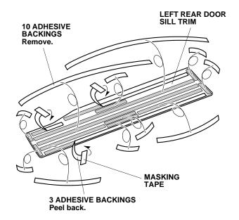
19. Remove the remaining adhesive backings.
