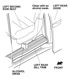
14. Attach masking tape to the left rear sill trim as shown.
