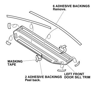
8. Remove the remaining adhesive backings.
