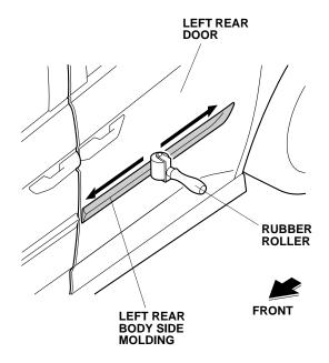
15. Turn the template over and repeat steps 1 through 14 to install the body side molding on the right side of the vehicle.
