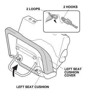
9. Lower the left seat cushion. Reinstall the two seat belt buckles into the loops.
