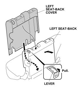
4. Fold the left seat-back fully forward. Pull the seat-back cover tight, and secure it to the left seat-back with nine hook-and-loop fasteners.
