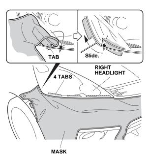
12. Pull the mask smooth, and secure the snap on the mask to the snap-screw. Attach the fourth plastic hook to the fenderwell.
