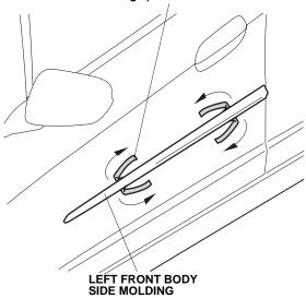
7. Using a rubber roller, apply firm pressure while rolling to set the adhesive.
