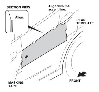
Peel back approximately 1½ to 2 inches of the adhesive backing, and tape the ends to the outer surface of the body side molding. Remove the small end pieces of adhesive backing.
