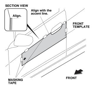
Peel back approximately 1½ to 2 inches of adhesive backing, and tape the ends to the front surface of the body side molding. Remove the small end pieces of adhesive backing.
