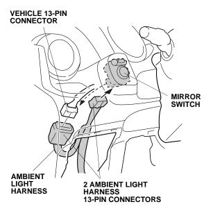
9. With accessory fog lights: Unplug the vehicle 13-pin connector from the fog light harness, and plug it to the ambient light harness 13-pin connector. Plug the other ambient light harness 13-pin connector into the fog light harness 13-pin connector.
