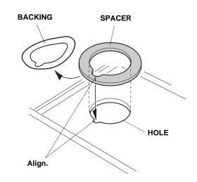
31. Align a grommet and shim through the hole as shown.
