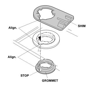
32. Attach the ambient light to the shim. Turn the ambient light clockwise to lock it in place.
