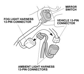
10. Using one wire tie, secure the excess ambient light harness and connector to the vehicle harness.
