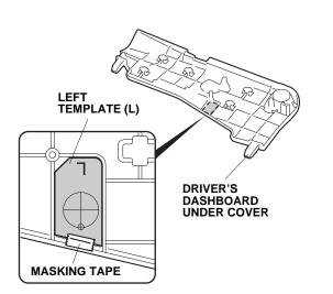
23. Using a pushpin, pierce the centers of the two scribe marks on the left template (L).
