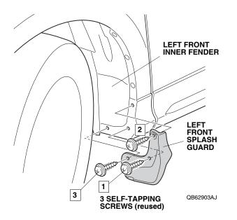
4. Turn the steering wheel fully clockwise, and repeat steps 2 and 3 to install the right front splash guard on the right side of the vehicle.
