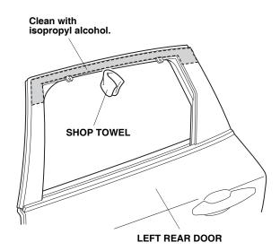
14. Peel back approximately 25–35 mm (1–1.5 inches) of adhesive backing, and tape the ends to the front surface of the left rear door visor.
