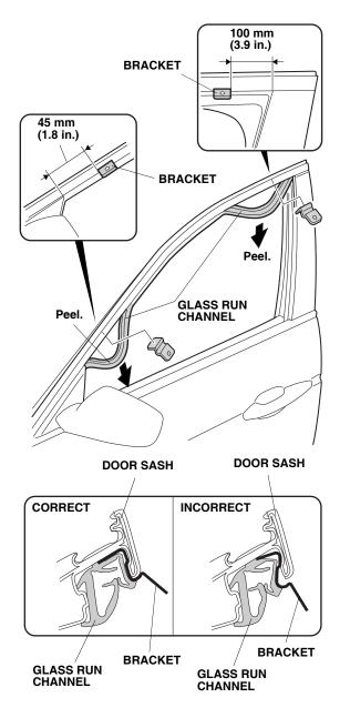
3. Install two brackets between the door sash and the glass run channel at the measurements shown. Then seat the glass run channel properly around the brackets.
