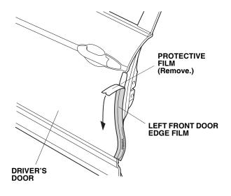
7. Starting from the middle of the door edge film and working outward, fold the left front door edge film around the edge of the driver's door using your fingers. Move your fingers in one direction. Attach the film over the seam sealant. Do not trim or damage the seam sealant.
