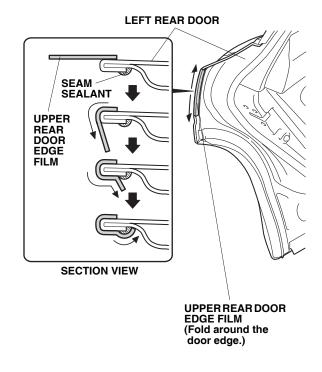
16. Using a lint-free shop towel, wipe the 3M protective tape application solution from the upper rear door edge film. Allow the upper rear door edge film to dry thoroughly.
