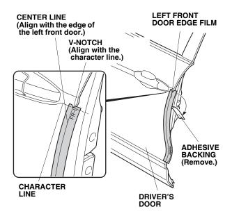
4. Continue to remove the adhesive backing while you align the center line of the door edge film with the edge of the door.
