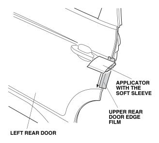
14. When you are satisfied that the upper door film is firmly attached to the edge of the door, slowly remove the outer protective film.
