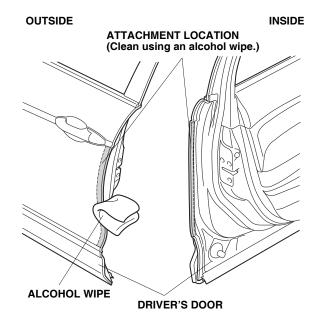
2. Close the driver's door. Using a spray bottle with 3M protective tape application solution, spray the area where the left front door edge film will attach.
