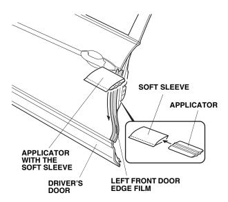
6. When you are satisfied that the door film is firmly attached to the edge of the door, slowly remove the outer protective film.
