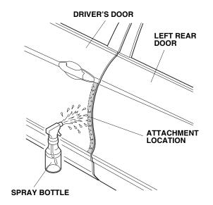
Open the driver's door again. Peel back about 50 mm (2 in.) of adhesive backing from the left front door edge film. Align the V-notch in the door edge film with the end of the character line on the upper part of the door.
