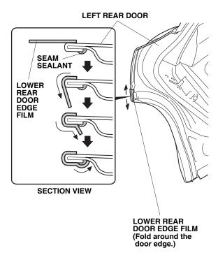
24. Using a lint-free shop towel, wipe the 3M protective tape application solution from the lower rear door edge film. Allow the lower rear door edge film to dry thoroughly.
