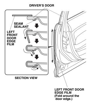
8. Using a lint-free shop towel, wipe the 3M protective tape application solution from the door edge film. Allow the front door edge film to dry thoroughly.
