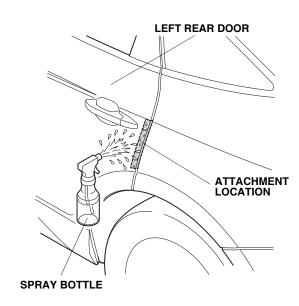
11. Open the left rear door again. Peel back about 50 mm (2 in.) of adhesive backing from the upper rear door edge film. Align the V-notch in the door edge film with the end of the character line on the upper part of the rear door.
