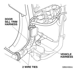
18. Continue to route the door sill trim harness along the vehicle harness, then loop the connector back to the measurement shown. Secure the door sill trim harness to the vehicle harness with one wire tie.
