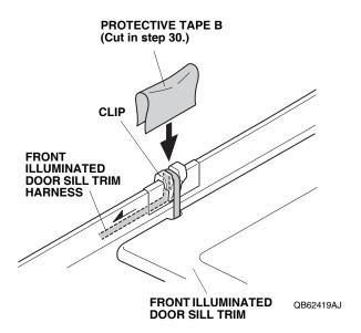
59. Plug the front illuminated door sill trim harness 2-pin connector into the door sill trim harness 2-pin connector.
