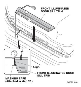
41. Attach the front illuminated door sill trim to the vehicle panel by removing three adhesive backings in the order shown and pressing on the trim firmly with your hands.
