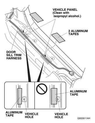
29. Secure the door sill trim harness to the vehicle panel with two aluminum tapes.Do not attach the aluminum tape over any vehicle
