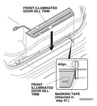
56. Attach the front illuminated door sill trim to the vehicle panel by removing three adhesive backings in the order shown and pressing on the trim firmly with your hands.
