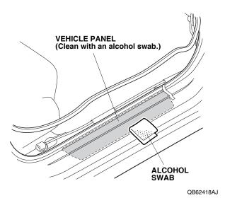
55. Position the front illuminated door sill trim on the vehicle panel and align it with the masking tape.
