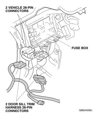
14. Attach the door sill trim harness 28-pin connector to the vehicle 28-pin connector.
