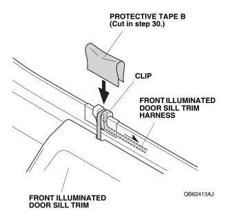
44. Plug the front illuminated door sill trim harness 2-pin connector into the door sill trim harness 2-pin connector.
