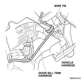
20. Secure the door sill trim harness to the holes in the dashboard panel with two wire ties. If another accessory harness is already attached to the dashboard panel, route and attach the other harness below the door sill trim harness.
