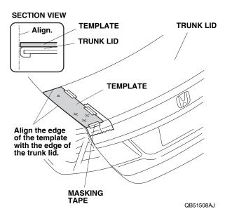
5. Using a felt-tip pen, mark the trunk lid through the template at the three locations shown on the template.
