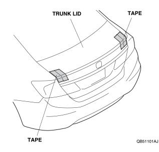
4. Place the template on the left side of the trunk lid, and align the template with the edge of the trunk lid as shown. Tape the template to the trunk lid with strips of masking tape.
