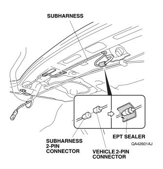
35. Align the green tape on the subharness with the vehicle clip, and secure the subharness to the vehicle harness with one wire tie.
