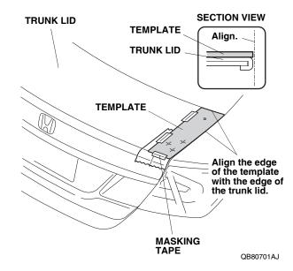
8. Using a felt-tip pen, mark the trunk lid through the two outboard in the template. Do not mark the inboard hole.
