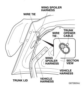
31. Route the subharness through the holes in the vehicle panel as shown.
