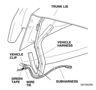
36. Connect two wire ties together and secure the subharness to the vehicle panel with the connected wire tie.
