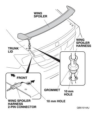
18. Remove two adhesive backings from the wing spoiler.
