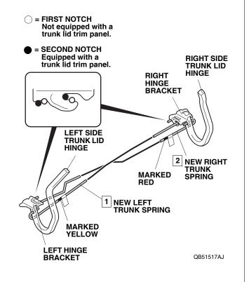
26. Reinstall the center clip to the trunk springs.
