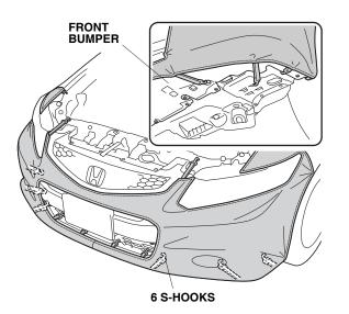
17. Route the elastic cord through eight loops on the bottom of the mask. Attach one S-hook to the bottom edge of the bumper on one side. Stretch out the cord after routing it through each loop, then attach the other S-hook to the bottom edge of the bumper on the other side.
