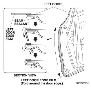
8. Using a shop towel, wipe the excess 3M protective tape application solution from the left door edge film. Allow the left door edge film to dry thoroughly.
