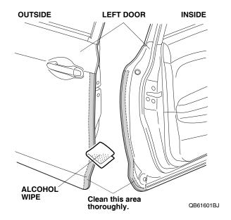
Close the left door. Using a spray bottle with 3M protective tape application solution, spray the outer area where the left door edge film will attach.
