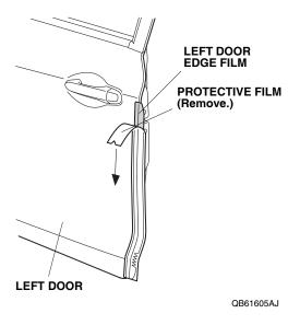
7. Starting from the center and working outward, use your fingers to fold the left door edge film around the edge of the left door as shown. Move your fingers in one direction only. Attach the left door edge film over the seam sealant. Do not trim or damage the seam sealant.
