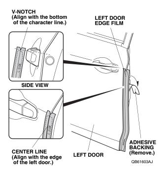
4. Align the center line on the left door edge film with the edge of the left door. While applying light pressure, carefully remove the adhesive backing, and attach the left door edge film to the left door.
