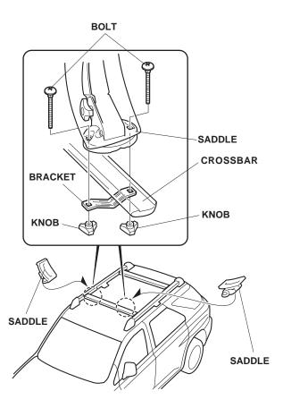
Position the two hydro-glide assemblies on the rear crossbar, and loosely install the hydro-glide assemblies using one bracket, two bolts, and two knobs for each assembly. The distance between the two assemblies should be the same width as the kayak.
