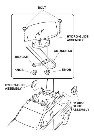
Rest the front of the kayak on the hydro-glide assemblies. Standing behind or alongside the kayak, lift up the rear of the kayak and push it forward, sliding it on the hydro-glide assemblies and saddles. Make sure the kayak reaches the front saddles before you lower it.
