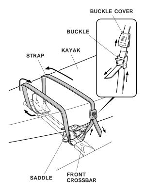
8. Route the strap from the buckle under the rear crossbar and around the kayak as shown. Slide the buckle cover away from the buckle, route the strap through the buckle, and tighten the strap. Slide the buckle cover back over the buckle.
