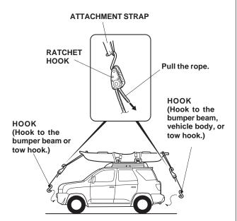
13. To loosen the rope, push up on the ratchet release lever, then pull on the rope.
