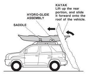
4. Adjust the distance of the saddles and hydro-glide assemblies to the same width as the kayak, then secure the saddle and the hydro-glide assemblies by tightening the knobs you installed in steps 1 and 2.
