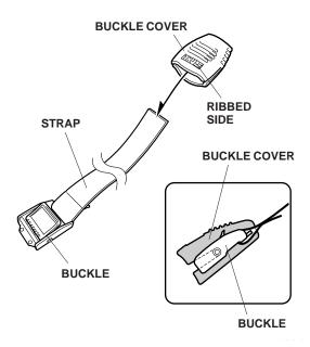
7. Route the strap from the buckle under the front crossbar and around the kayak as shown. Slide the buckle cover away from the buckle, route the strap through the buckle, and tighten the strap. Slide the buckle cover back over the buckle.
