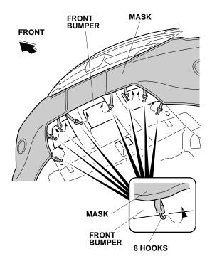
5. On each side, attach one hook to the hole in the front bumper.
