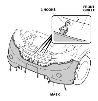
3. On each side, insert six tabs between the headlight and the grille.
